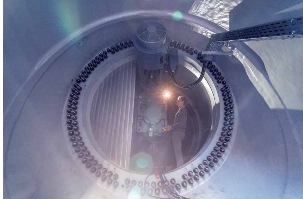
— Superlative rotor bearings: weighing 14 tons and so large that people can walk around in them. — These are the dimensions of rotor bearings for wind turbines.
