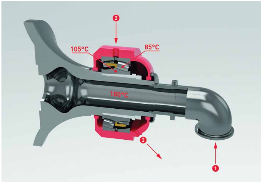
— Example of a dryer cylinder roll structure showing the typical temperatures present. 1 Steam, 2 Lubrication oil, 3 Oil return
