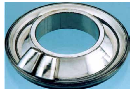
— Fig. 9 - Bearing failure due to improper mounting. The bearing was installed while magnetized
