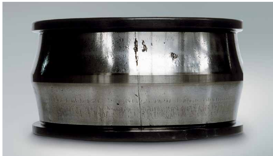
— Fracture evident on the through-hardened inner ring of a spherical roller bearing due to hoop stress
