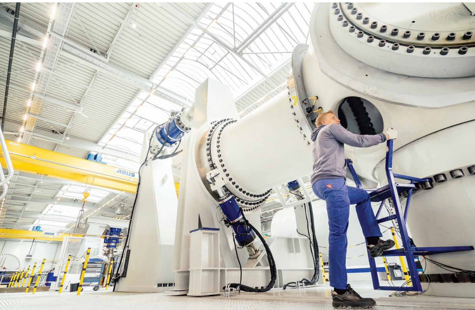
— Highly complex production: Since 1998 thyssenkrupp rothe erde in Lippstadt has been developing and producing rotor bearings for various types of wind turbines.
