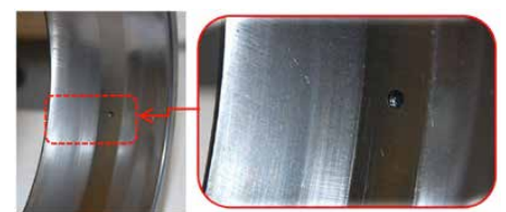
— Fig. 3 - Abrasive wear on the outer ring raceway surface of a spherical roller bearing
