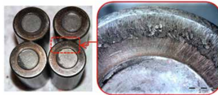
— Fig. 8 - Smearing of cylindrical roller end face
