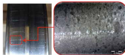
— Fig. 12 - False brinelling at the roller pitch identified on the spherical roller bearing inner ring raceway
